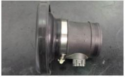
11.b. Place the second rubber boot on the other end of the MAF tube at an angle of 45 degrees. Secure with a 91-114mm hose clamp.
