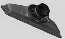
11.f. Insert the duckbill drain and 2 grommets into the bottom front half of the OTR.
