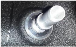
18.a. Fit the MAFless rubber boot to the rear section of the OTR as shown. 18.b. Secure with the 105-176mm hose clamp.
