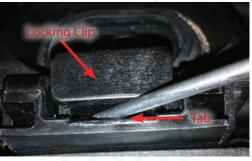
2.b. Using a flat screw driver, place it in the slot inside the top mount and lever the ratchet tab away far enough to unlock it and wiggle the mount upwards and remove.
