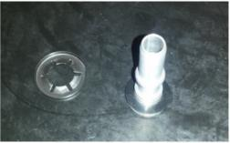
17.c. Push the fitting through the rear section of the OTR. 17.d. Use the 12.7mm push on clip to secure the breather fitting in place. ( A socket can be used to assist pushing the locking clip on.)
